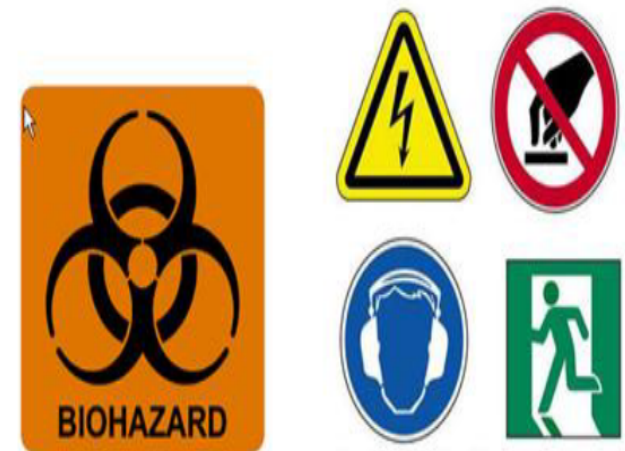
Figure 2. ISO 3864 safety sign formats (clockwise from top left): warning sign, prohibition sign, mandatory action sign, and safety information sign.
